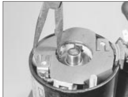
22.10 Using pointed-nose pliers to compress the brushes
